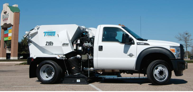
The Model 210h® delivers great sweeping performance in a "single engine" class design. With the Ford Super Duty F-450, the Model 210h has a tight turning diameter of 44.2 feet, and overall height of 80.5 inches. The Ford F-350 turning diameter is 50.8 feet, and has an overall height of 78 inches, perfect for sweeping in parking garages.
